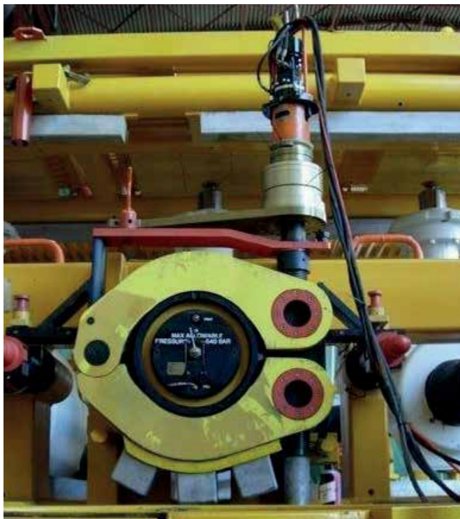
Wet Pipe Clamp Tool under test
