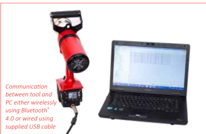
Built in Bluetooth® for wireless data transfer
